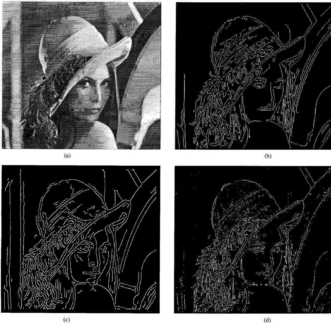
Fig. 5. Comparison of the edge detection results on the Lena picture. (a) Input intensity image. (b) Detected edges by the proposed 2-D edge detection functional Q_{edge} with \sigma = 2.5 . (c) Detected edges by the 2-D Canny edge detector with \sigma = 2.5 . (d) Detected edges by the Marr-Hildreth edge detector with \sigma = 2.5 .
