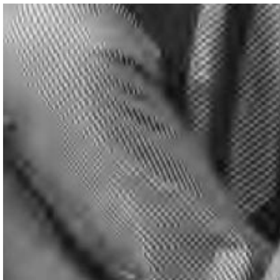
Fig. 9. Barbara at 0.25 bpp (corresponds to a 32:1 compression ratio) with Bi22/14 wavelet; PSNR = 26.85 dB.
