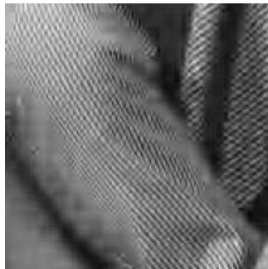
Fig. 10. Barbara at 0.25 bpp (corresponds to a 32:1 compression ratio) with BSA9/7 multiwavelet; PSNR = 26.80 dB.
