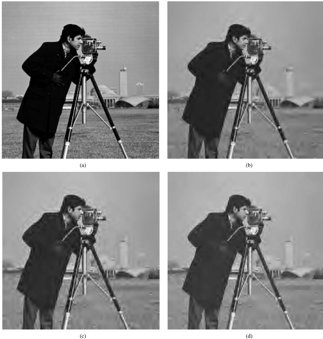
Fig. 13. Cameraman image compressed to 0.25 BPP (32:1 compression). (a) Cameraman image. (b) Compressed with Daubechies (9,7). (c) Compressed with linear (1,7) lift. (d) Compressed with adaptive lift.
