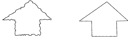
Fig. 4. A noisy polygonal contour and the corresponding most stable polygon.
