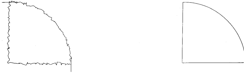
Fig. 7. For this jagged quarter circle, the only stable shape is the one with two straight parts and one curved part. The estimated tangents are drawn directly on the original noisy contour to the left and to the right is the final approximation.
