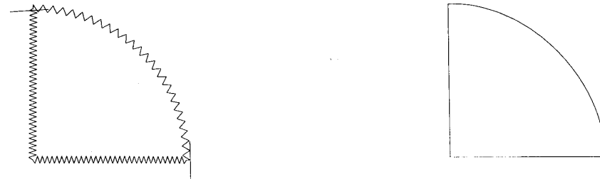
Fig. 8. A slightly different version of the same pattern. Again good tangent estimates are found. We note that our algorithm has not chosen the corner breakpoints symmetrically. The top-left corner is on the inside of the curved part and the bottom-right corner is on the outside.
